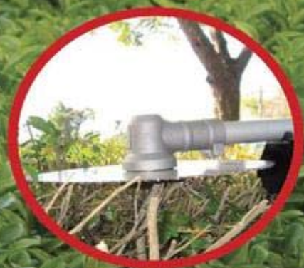
90° Heavy Duty Alum. Gear case ass'y applied with Tip Saw 100T Blade (10")
